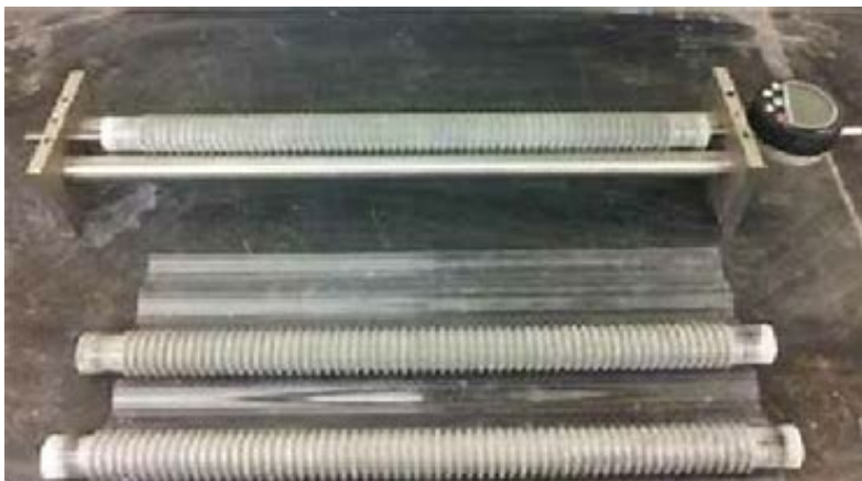
Figure 6: ASTM C1698 Autogenous Shrinkage (All photos provided by FHWA Federal Lands)
